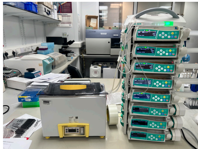
Figure 1 Set-up of laboratory transfusions using syringe pumps, lines and water bath.
