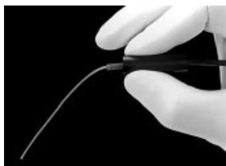
Figure 1 Probe microphone/tube used to measure noise intensity.
