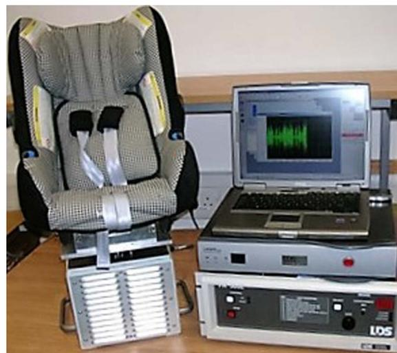
**Figure 1** Car seat motion simulator with controls.
