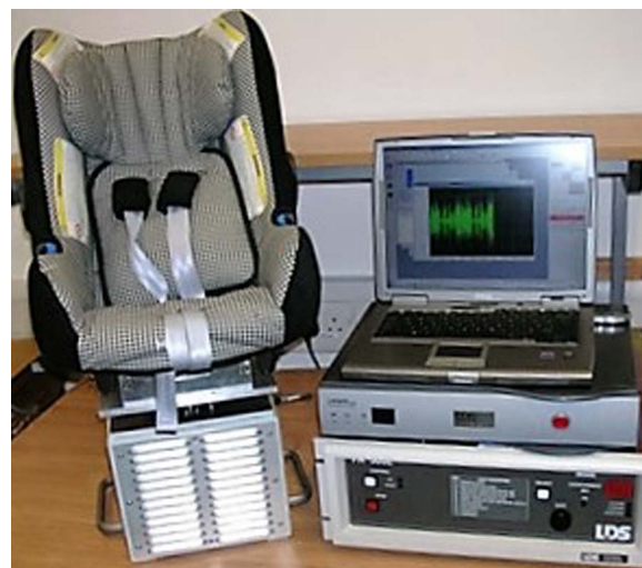
Figure 1 Car seat motion simulator with controls.
