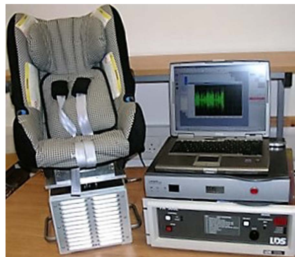
Figure 1 Car seat motion simulator with controls.
